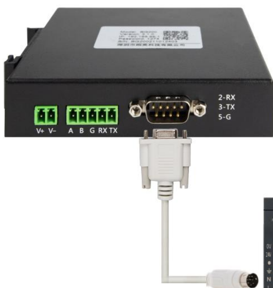
DB9 232 to round eight-pin 232 communication line
